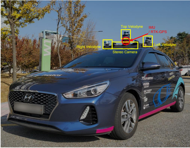
Fig. 6. In-house dataset MMS platform. Our platform contains triple 16-ray LiDAR (Velodyne VLP-16), MEMS-IMU (Xsens MTI-30G), stereo camera (FLIR BlackFly S) and RTK-Level INS integrated GPS (Ublox ZED-F9K).
