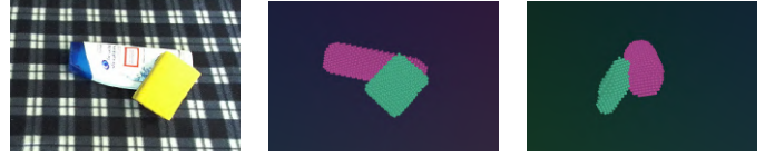
Fig. 7: Object-aware and holistic scene understanding. Given the input image (left), CenterGrasp is able to predict a full per-object reconstruction even in the presence of partial occlusions (center-right).
