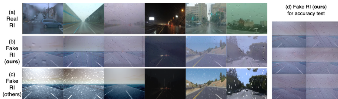
Fig. 6. Comparison between Real and Fake Rainy-Images. (a) Rainy-Images in actual road rainfall conditions (b) Rainy-Images created using our method (c) Rainy-Images produced by methods of Hendrycks et al. (2019), Tremblay et al. (2021), and Jeon et al. (2022) (d) Fake Rainy-Images generated by adjusting parameters such as n_{arc} , \alpha for accuracy testing.
