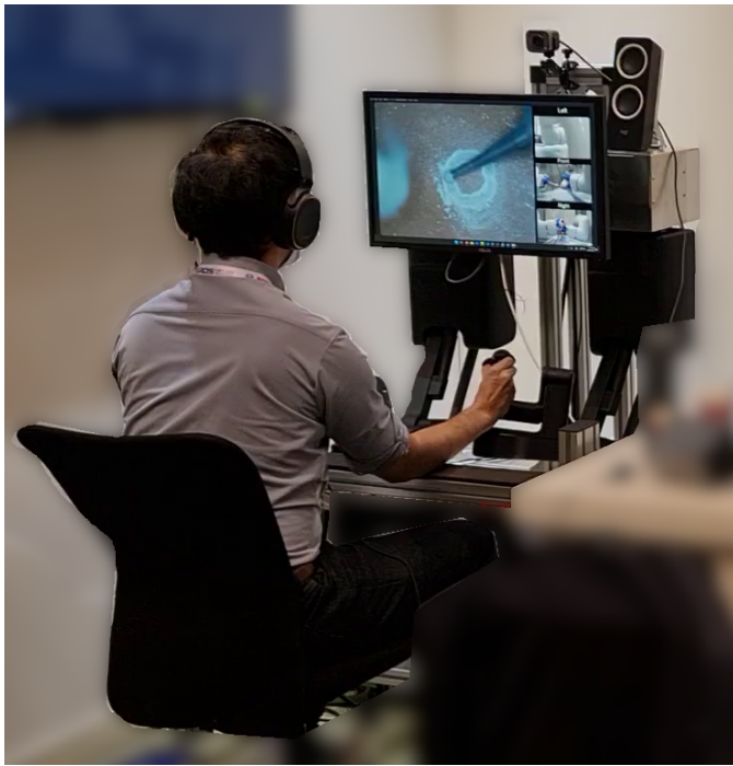
Fig. 6. Kyoto-side operator console. The operator had access to two control interfaces similar to those used by the Hinotori surgical robot system. The user had a view composed of the Tokyo-side microscopic image taking most of the screen and three smaller views on the right corresponding to the left, front, and right views of the Tokyo-side system. In addition, the operator could hear the drilling sounds using speakers.
