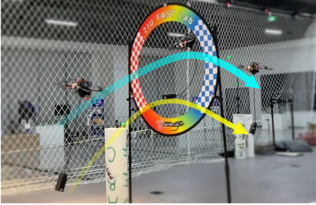
Fig. 1. Quadrotor with a cable-suspended payload successfully navigates through a narrow circular gate, demonstrating natural mode-switching movements in the suspended payload system.
