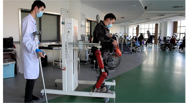
Fig. 1: A patient is gait training with an exoskeleton robot associated with a robotic walker, where the weight of the human-exoskeleton system can be supported by the walker.
