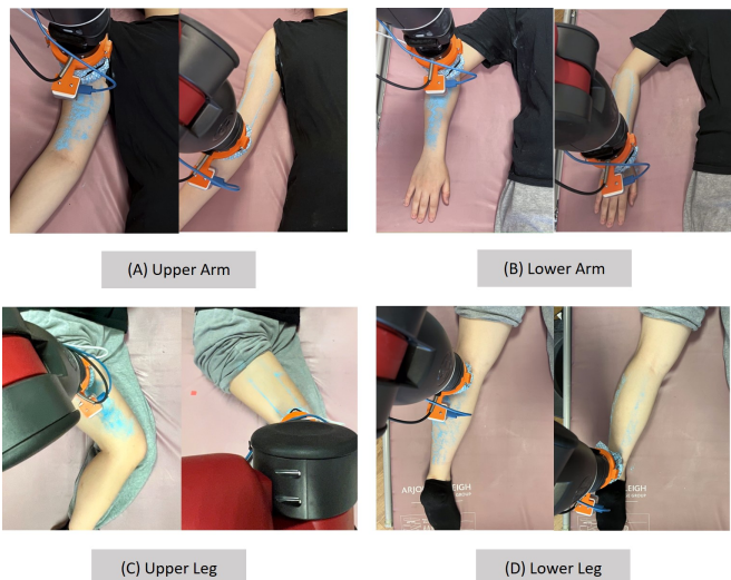
Fig. 8. Snapshots of Baxter robot providing bathing assistance to a real human for four body parts. The example trials are also provided on our project website.
