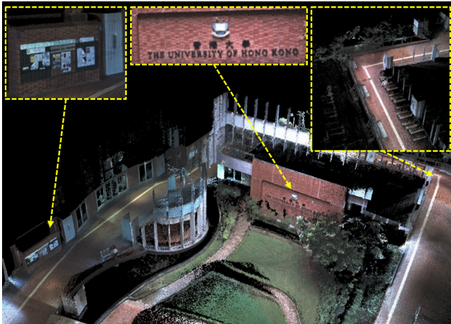
Fig. 5. Our SR-LIVO is able to reconstruct a dense, 3D, RGB-colored point cloud map, which is comparable to the reconstruction result of R3Live (Fig. 1 in [5]).
