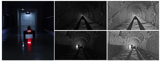
Fig. 6. Left : Dark indoor long corridors - challenges include illumination changes and straight long corridors. Middle, Right : Underground mine - challenges include poor lighting conditions, straight long tunnels, self-similar areas, and low texture. The Middle is the original gray image, and the Right is the enhanced image.
