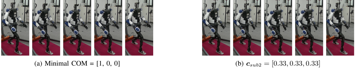
Fig. 1: Right leg lunge motion snapshots of HRP-4J for some combinations of weights of objective functions. The robot bends to lower its upper body and then gradually returns to its initial posture.
