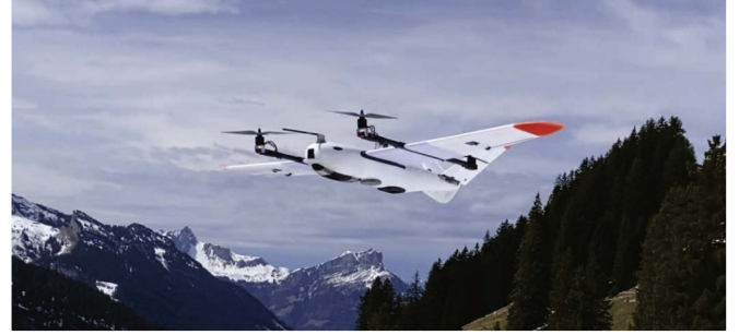
(a) Tiltrotor VTOL platform in flight during take off in Riemenstalden, Switzerland.
