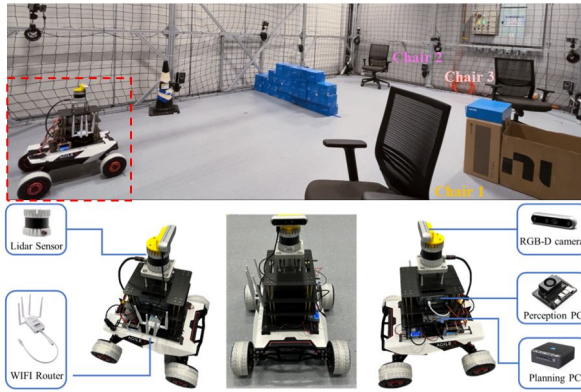
Fig. 7: (Up) The multi-room environment. The wheeled vehicle used is enclosed in the red dashed box. (Down) The details of the wheeled vehicle used in real-world experiments.
