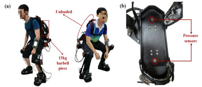
Fig. 8. Actual photographic: (a) Experiments on the motion of the PTEXO robot with and without load. (b) Installation site for plantar pressure sensors.
