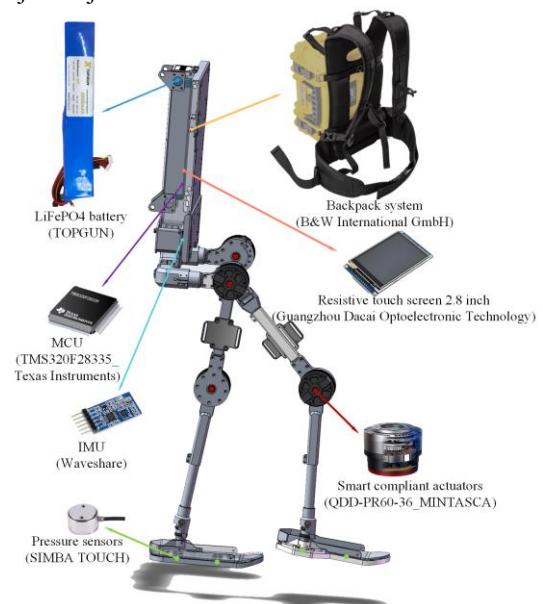
Fig. 1. PTEXO's electronic control hardware deployment scheme.
