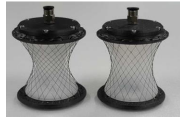
Fig. 2 Prototype of hyperboloidal pneumatic artificial muscle (h-PAM).
