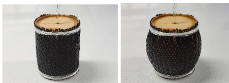
Fig. 17 Contraction behavior of a McKibben actuator (0 to 50 kPa).
