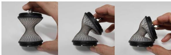
Fig. 18 Bending test demonstrating the flexibility of the muscle.
