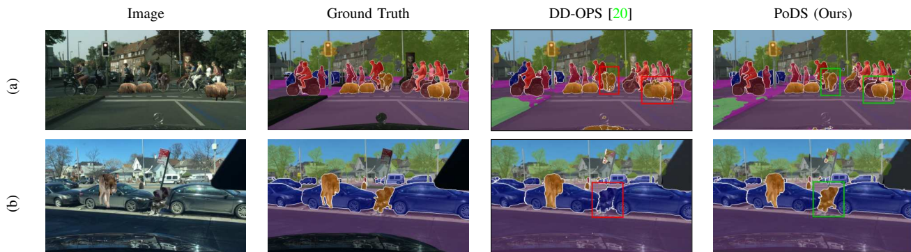
Fig. 9: Qualitative panoptic out-of-distribution segmentation results of our proposed PoDS network in comparison to the state-of-the-art baseline DD-OPS [20] on (a) Cityscapes-OOD and (b) BDD100K-OOD datasets. Red boxes highlight regions with errors in the segmentation, while the corresponding green boxes indicate regions with correct segmentation.
