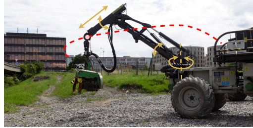
Fig. 11. A picture of SAHA with the controllable joints marked in yellow. The red circle shows the mounting point of the underactuated cutting tool. In the experiments, we control the active cylinders on the arm to track task space trajectories (red dashed line) with the tool mounting point.
