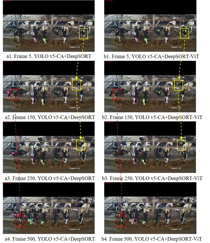
Fig. 4. Comparison of YOLOv5s-CA+DeepSORT and YOLOv5s-CA+DeepSORT-ViT tracking results. The red box tracking is the cow ID7 recognition and tracking effect, and the yellow box tracking is the cow ID4 recognition and tracking effect.
