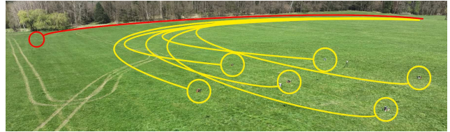
Fig. 1: A swarm of six UAVs (yellow) tracking an intruder drone (red) using the proposed approach. The group velocity of 5 \text{ ms}^{-1} was reached, while the swarm stayed coherent without reliance on GNSS and communication. Circles show the positions of UAVs at the beginning of the experiment.
