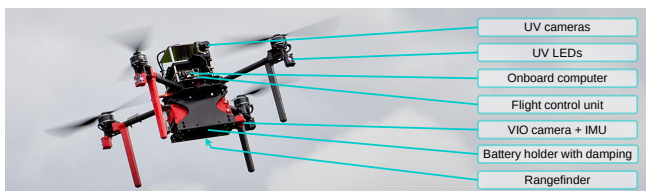
Fig. 5: Hardware setup of UAVs used in experiments.
