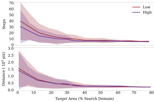
Fig. 9: The performances of the Lissajous-based heuristic method under two different visibility levels. In environments with low soil level, the agent on average took only 10 more steps to locate targets with low visibility than with high visibility.
