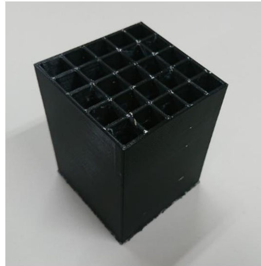
Figure 2. Photograph of a container fabricated to prevent the roots of pea sprouts from entangling with each other during hydroponic cultivation. This is compartmentalized for each pea sprout. Part of the top is closed just enough to allow the roots to pass through to hold the seed in place.
