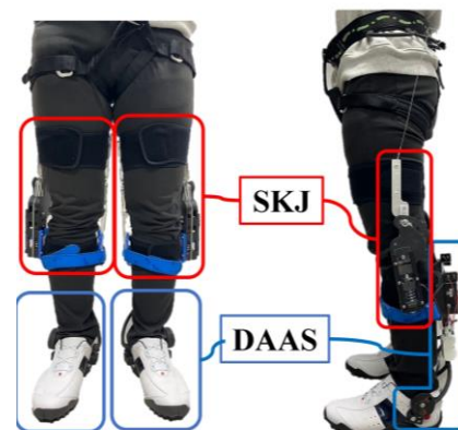
Figure 1. Biomimetic Assist Suit (BAS)
