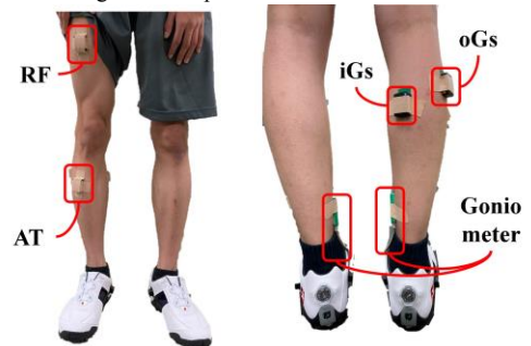
Figure 13. Position of EMG sensors and Goniometers
