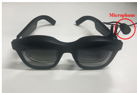
Fig. 1. Smart glasses that perform sound analysis in real time and output the results on the lens to enable visual recognition of detection results.
