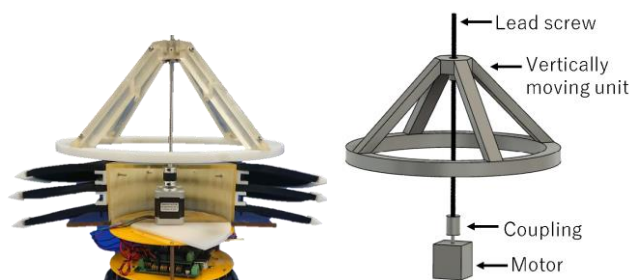
Figure 6. Lock/unlock unit of the omni-directional robot.
