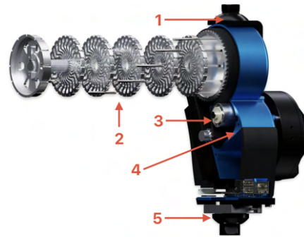
Fig. 1. OSL 2.0 Knee Joint [6]. 1: Knee Connector with Pyramid Adapter, 2: Serial Elastic Actuator Output Pulley, 3: Belt Tensioner, 4: Housing, 5: Loadcell & Pyramid Adapter
