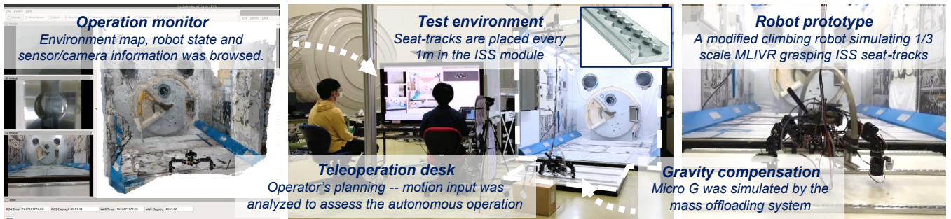
Fig. 2: Concept of operation: preliminary testing to demonstrate a real operation from the ground to the space station ©JAXA/Tohoku Univ. Space Robotics Lab.
