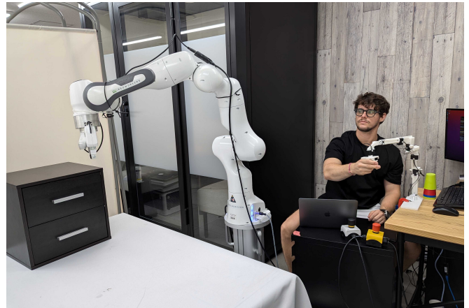
Fig. 1: The low-cost GELLO teleoperation system (right), controlling a Franka Panda 7 DoF robot arm (centre).
