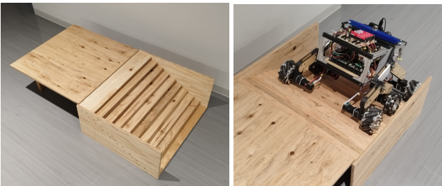
Figure 7. Experimental environment.(a. stairs ID24-48, b. Rocker-bogie on the stairs ID12-24)
