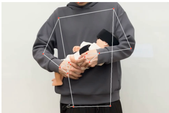
Fig. 3. Posture estimation with MediaPipePose
