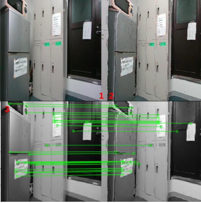
Fig. 5. Scene generation and matching : 1: image after traveling 2: generated scene on position and pose where odometry indicates 3: matching two scenes with SIFT algorithm
