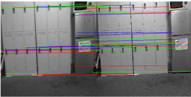
Fig. 11. SIFT Matching result: Left(Drone's camera image), Right(Generated image by the Renderer)
