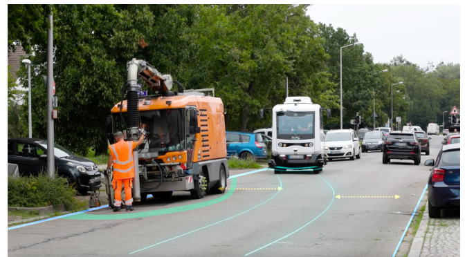
Fig. 1: The EVA shuttles Ella, Vera, and Anna have been deployed in a peri-urban area of Karlsruhe. The shuttles choose their movement freely between road boundaries and breaking free from the virtual rail. The steering wheel-free shuttles keep the automated distance from sensed obstacles and, if necessary, drive onto the opposite lane.
