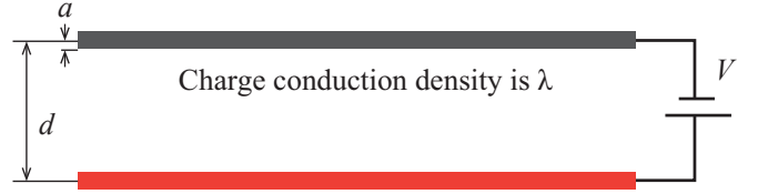
Fig. 2. Two conductive threads with an applied potential difference
