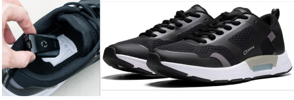
Fig. 1: ORPHE smart shoes with in-shoe IMUs [9]
