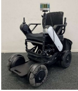
Fig. 1 The Personal Mobility Tool (PMT) used as the autonomous electric wheelchair in this study.
