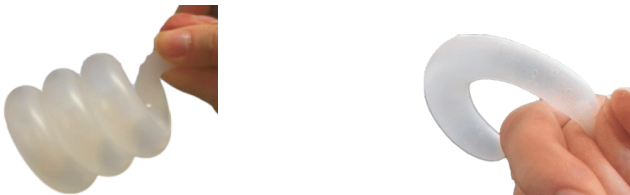
Fig. 4. Two fully inflated tentacles with single material and off-axis air channel. Ecoflex, with its higher tensile strength enables a neat spiral shape (left) and Dragon Skin due to its higher stiffness formed into a rainbow shape (right).
