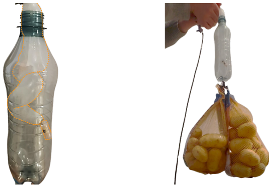
Fig. 12. Grasping method C with a 50% Ecoflex and 50% Dragon Skin tentacle. The tentacle is placed inside a bottle to test its gripping and load-bearing capabilities. (Left) When inflated to a differential pressure of 338 kPa, the tentacle curls, creating multiple contact points with the neck and inner surface of the bottle. (Right) The tentacle grips the bottle from the inside, holding a 5 kg load while the experimenter lifts only the tentacle.
