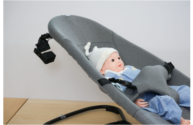
Fig. 1. Detachable robot that moves the baby bouncer
