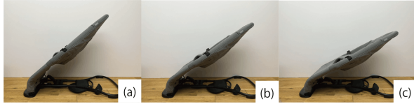
Fig. 3. Three types of baby bouncer inclination: (a)High, (b)Middle, (c)Low
