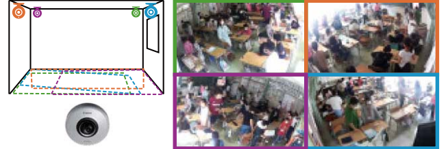
Fig. 5. Layout of the camera system
