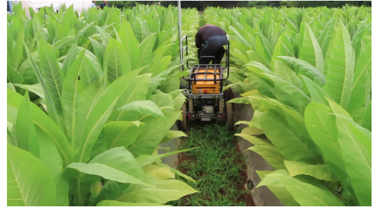
Fig. 1: Scene of agricultural robot assisting with harvest transport by following worker
