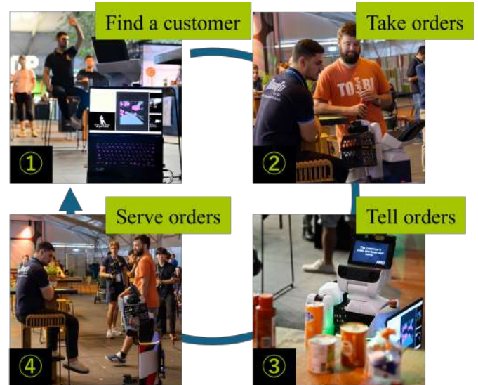
Fig. 1: “Restaurant” task in Robocup@Home
