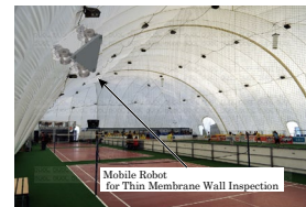
Figure 2: Basic concept of the mobile robot for environments with membrane structures [14].
