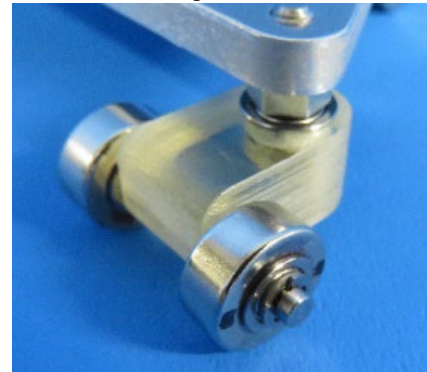
Figure 5: A single unit of the magnetic twin-caster mechanism.
