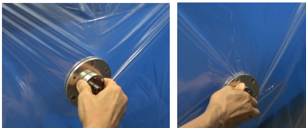
(a) Major deformation in the form of wrinkles (b) Film damage caused by sliding contact
