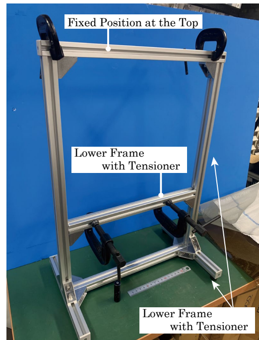
Fig. 18: Experimental Setup for Wall Climbing with Different Tensioner Sheets
