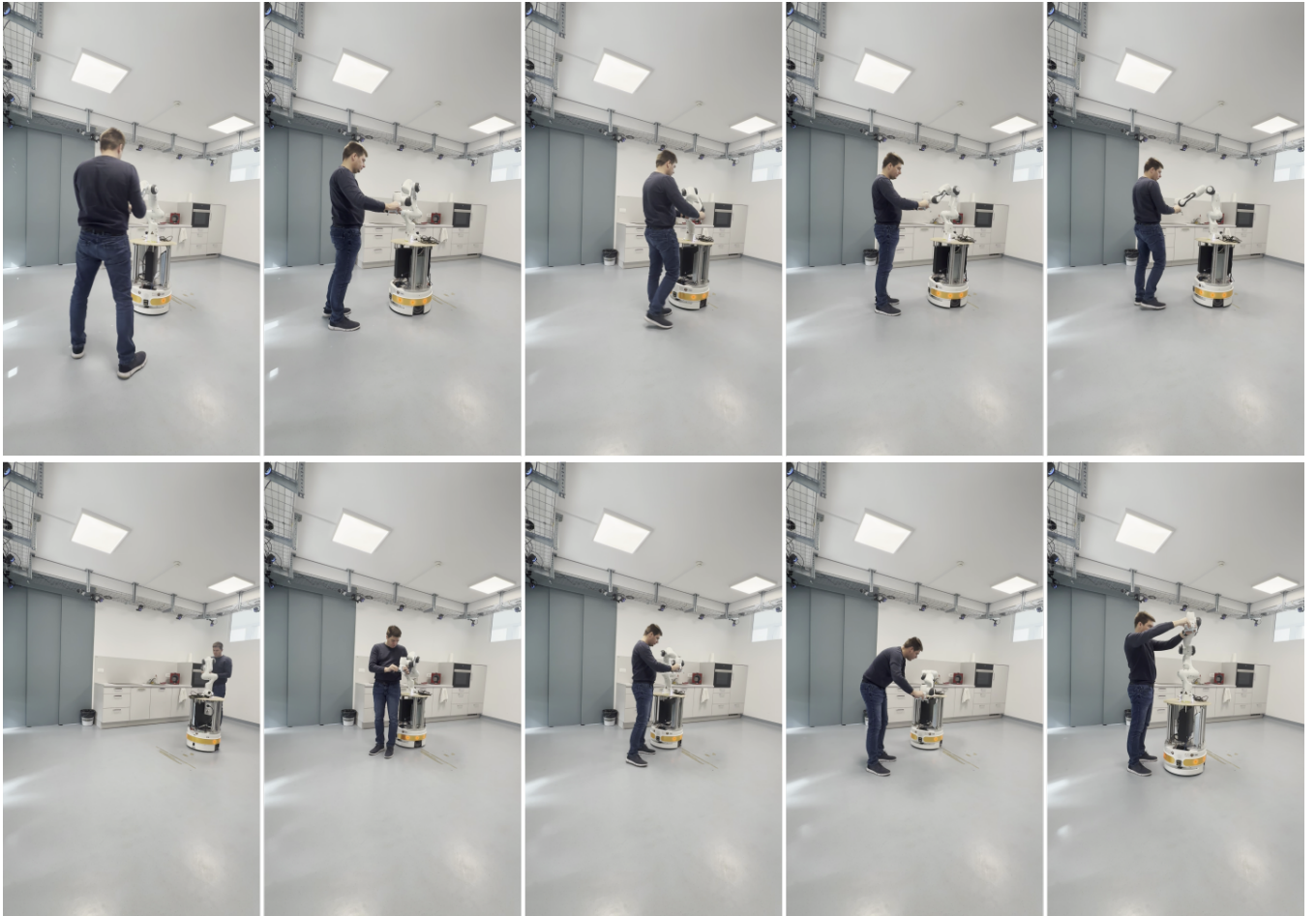
Fig. 4: Sequence of kinesthetic guidance. As the operator physically moves the robot arm, the mobile base responds automatically by following the end-effector to maintain manipulability. This sequence corresponds to the experimental demonstration shown in Supplementary Multimedia 1.
