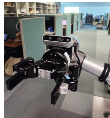
(c) End-effector-mounted Intel Realsense D435i at an angle of 45°.
