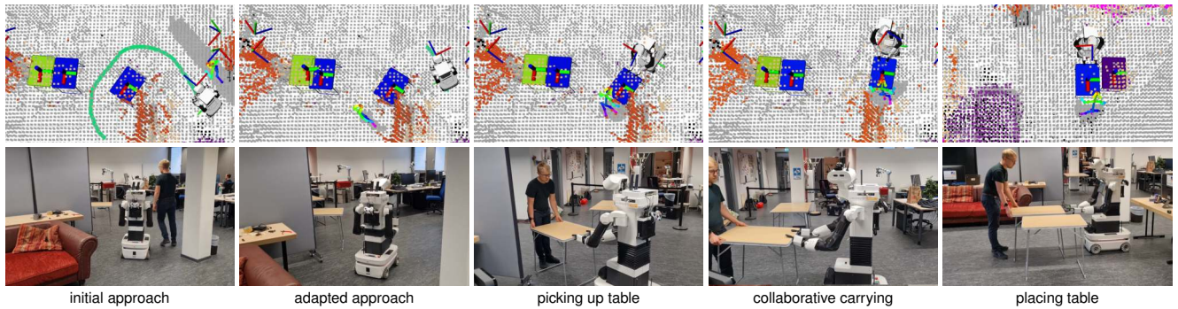
Fig. 8. Collaborative table carrying task. The robot anticipates the person’s choice of which table to carry and which side to grasp. The person guides the compliant robot via interaction forces through the table. The robot anticipates the target placement location and takes the lead for precise positioning.
