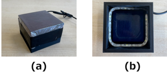
Fig. 2. (a) The sensor module developed in this paper. (b) The internal state of the sensor.
