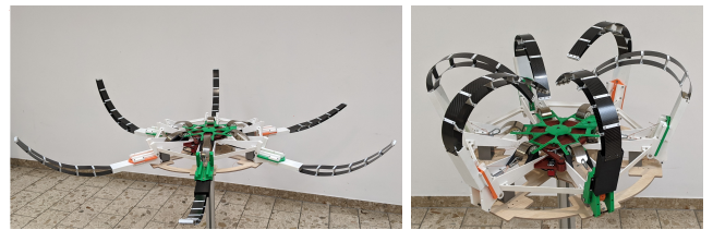
Fig. 9. Working prototype of the gripping system with a 180° opening angle. Left: open state; Right: closed state.
