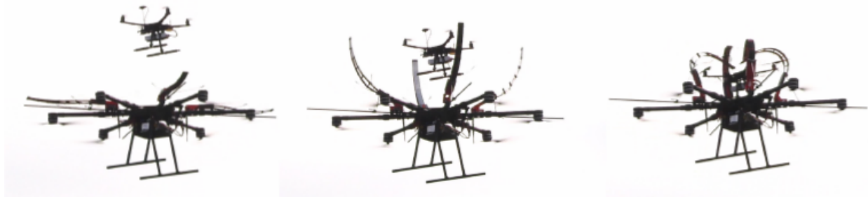
Fig. 12. First manual flight test with gripping system.
