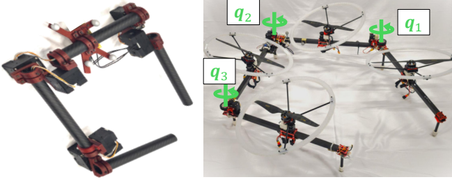
Fig. 6: Left: Snapshot of the teleoperation device. Motion capture markers are attached to measure position and attitude. Servo motors are attached to each joint to measure roll and pitch joint angles. Right: Snapshot of HYDRUS_XI, the articulated aerial robot to be teleoperated. It has three joints ( q_1 , q_2 , q_3 ) that rotate in the yaw direction.
