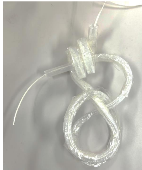
Fig. 9 Test results of the lacing tape passage using the hose-shaped mold.
