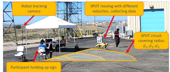
Fig. 1. Experiment setup to assess reliability of hand gesture recognition from a mobile robot, varying distance and viewing angle of a subject's hand from the mobile robot. A stabilized vision system mounted on the robot tracks and collects images of the subject as the robot moves over a prescribed path. The images are processed to infer hand sign as a function of distance and viewing angle of the hand from the robot.
