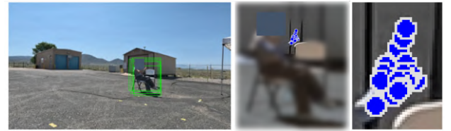
Fig. 8. Hand landmark detection from the SPOT is achieved by first detecting the participant. The cropped human frame is used to detect the hand landmarks.
