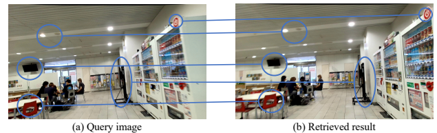
Fig. 12. Loop closure retrieval performance (AnyLoc LC). A large number of correspondences are detected between the two images, and a subset of them is highlighted. These matched keypoints are subsequently used for registration and pose graph optimization.
