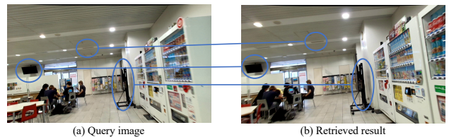
Fig. 13. Loop closure retrieval performance (Classical LC). The figure displays the query image and its matches, with similar feature regions highlighted. Although the most similar images are obtained by adjusting the threshold, the number of matched keypoints is insufficient and fails geometric verification.
