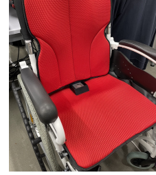
Fig. 2. Measurement method using illuminance sensor, one illuminance sensor in the center of the rearmost part of the seat of the wheelchair.
