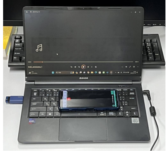
Fig. 3. Experimental setup showing the PC playback and smartphone recording arrangement.
